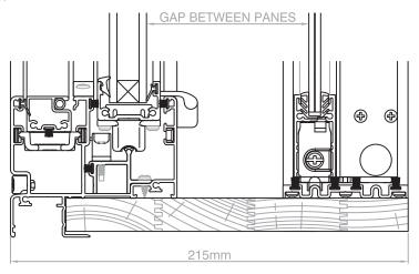
The custom lock body & dust cover hinges are cast in stainless steel & have a brushed finish
