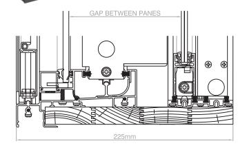
By spacing the secondary glazing away from the exterior frame, a gap between glass panes of around 100mm is created. In comparison to double glazing for thermal benefits, acoustic double glazing requires a much larger gap between each of the two glass panes
