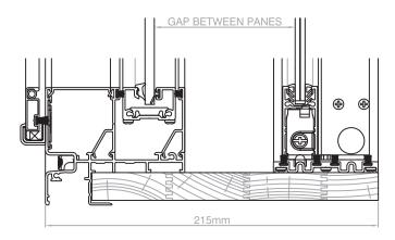
After-market or retro-fit systems often look like an obvious addition to the existing window. Acoustic Series products integrate both primary & secondary window elements inside the one reveal box, making for an attractive solution for noise attentuation
