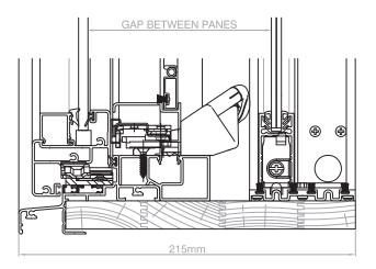
By spacing the secondary glazing away from the exterior frame, a gap between glass panes of around 100mm is created. In comparison to double glazing for thermal benefits, acoustic double glazing requires a much larger gap between the individual glass panes
