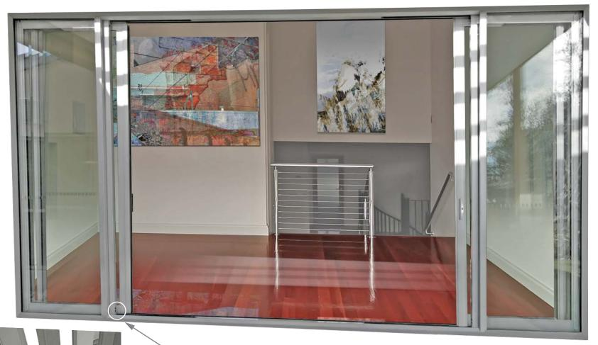
All panels roll on two 100kg rated, ball-bearing carriages which run on anodised track inserts
