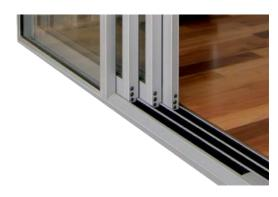
Each of the three rows of panels roll on two 100kg rated, ball-bearing carriages, which in-turn run on heavy-duty anodised track inserts. With the outer frame 200mm in depth, fly screens are unfortunately not possible
